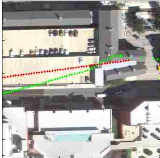
Figure 14: GPS multi-path causing a persistent error in GPS heading. The wheelchair is traveling West to East on the sidewalk South of the parking garage. The GPS has slowly drifted North and pulled the estimated position into a building. Such an error is almost indistinguishable from good data.
