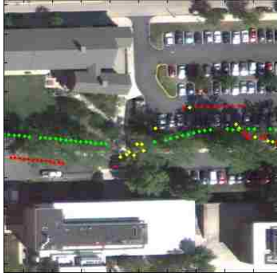
Figure 13: Particularly bad GPS data. The wheelchair is moving West to East on the sidewalk under trees. GPS fix is shown in red, rejected GPS fix is shown in yellow, the result of the EKF is shown in green. Notice that a multi-path error is not filtered because rotational velocity matches that of the wheelchair.
