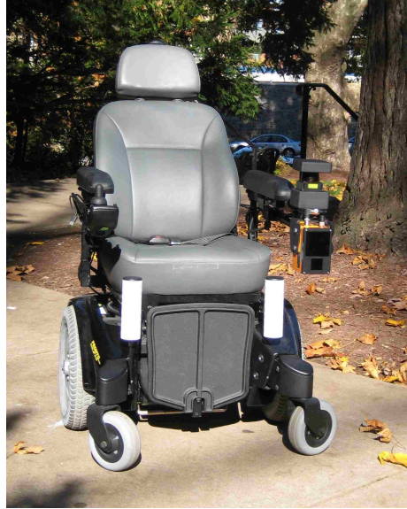
Figure 2: The smart wheelchair development platform integrates encoders, an 3DM-GX1 IMU, IFM O3D200 flash LIDAR, and WAAS enabled GPS.
